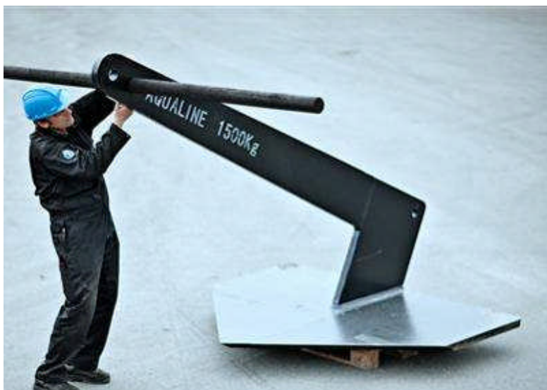
Figure 37: Frame or grid mooring using shovel anchors. Expensive design but feasible on deeper sites saving mooring rope
