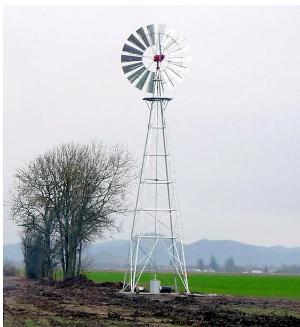
Figure 33: Windmills are first of all being used for pumping of water. Picture is showing an Ironman windmill from USA
